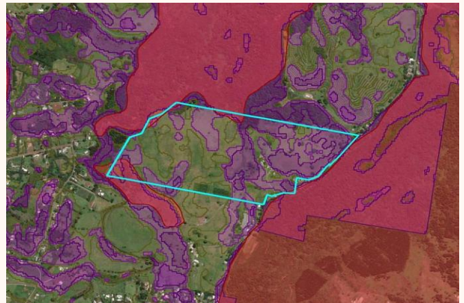
Landslide &amp; steep slope — landslide high ~5%; Cat 4 ~22%; Cat 3 ~28%.
